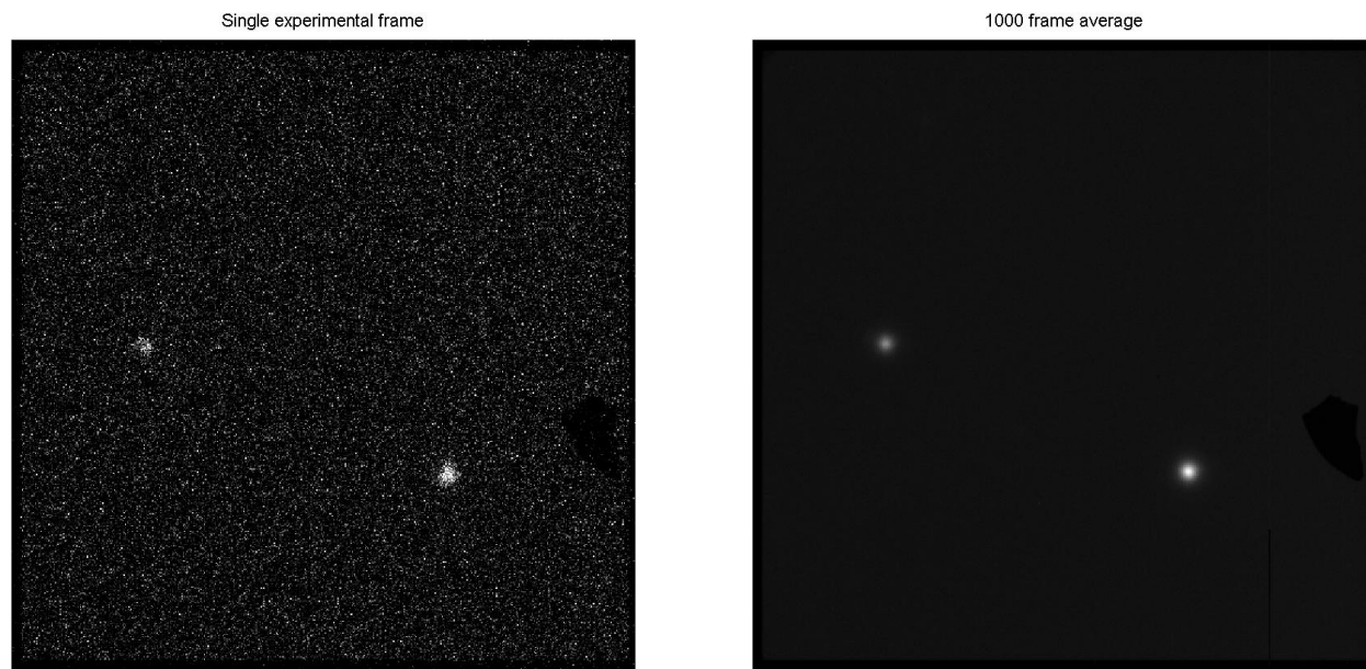
Figure 2. Experimental EMCCD frames. Left: Single experimental frame. Right: Average over 1000 individual frames. Where black = 0 photon/pixel/frame and white = 6.67 photons/pixel/frame
