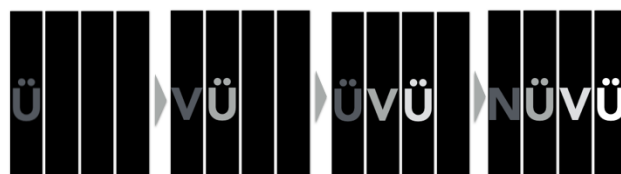
Fig. 1. Example of imaging the word NÜVÜ using Time-Delay Integration readout mode. The intensity of the signal is increased as the word moves across the detector.
